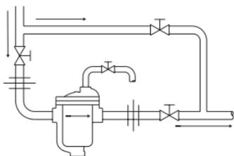
**Fig. 5-1.** Bypass hookups for No. 800-816 and 880-883 traps.
