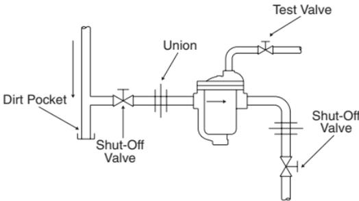
**Fig. 3-1.** Standard hookup No. 800-816, 800-883 traps, with shut-off valves to isolate trap during testing, inspection or repair. Unions should be at right angles—not in-line—to facilitate trap removal.
