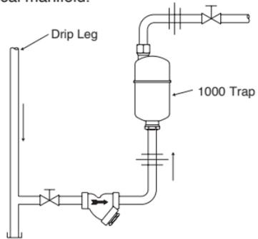
**Fig. 4-3.** Hookup for No. 1000 Series Stainless Steel trap.
