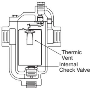
**Fig. 19-2.** Internal check valve installed in trap inlet.
