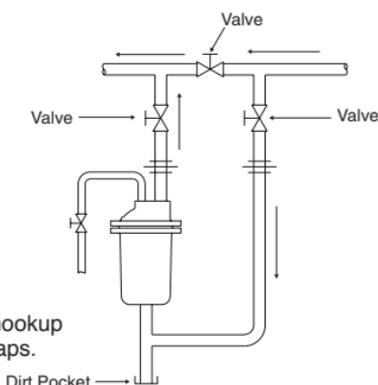
**Fig. 5-2.** Bypass hookup for No. 211-216 traps.
