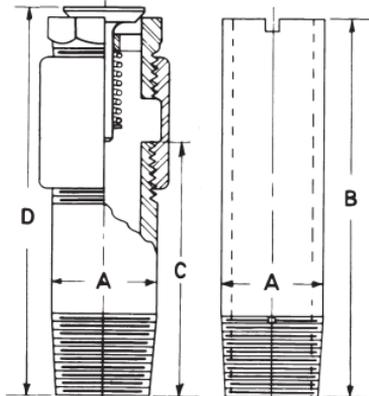
Tube with check valve and coupling.
