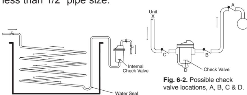
Fig. 6-1. Trap draining syphon.
