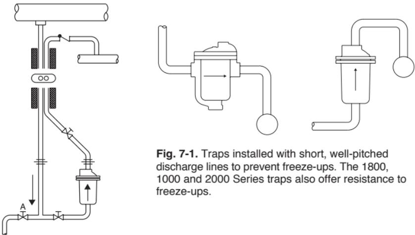
**Fig. 7-1.** Traps installed with short, well-pitched discharge lines to prevent freeze-ups. The 1800, 1000 and 2000 Series traps also offer resistance to freeze-ups.
