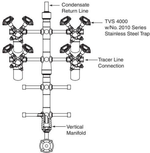
**Fig. 4-1.** Hookup for vertical manifold.
