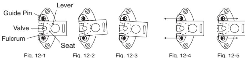
**Fig. 12-1** shows CORRECT ALIGNMENT of guide pins. When correctly aligned, lever can be moved sideways the same distance to the right (**Fig. 12-2**) as to the left (**Fig. 12-3**).
