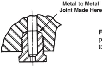
**Fig. 10-1. Important!** Valve seat seal is made at point of contact indicated, not by threads. Be sure to read paragraph above.
