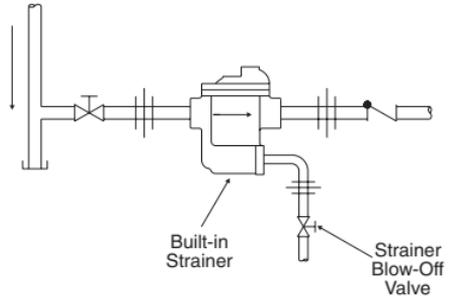
**Fig. 3-4.** No. 880-883 with strainer blow-down valve.
