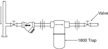
**Fig. 4-2.** Hookup for No. 1800 Series Stainless Steel trap.
